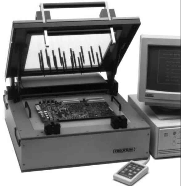
Model TR-7-3000-QC Lid Open to Install UUT
