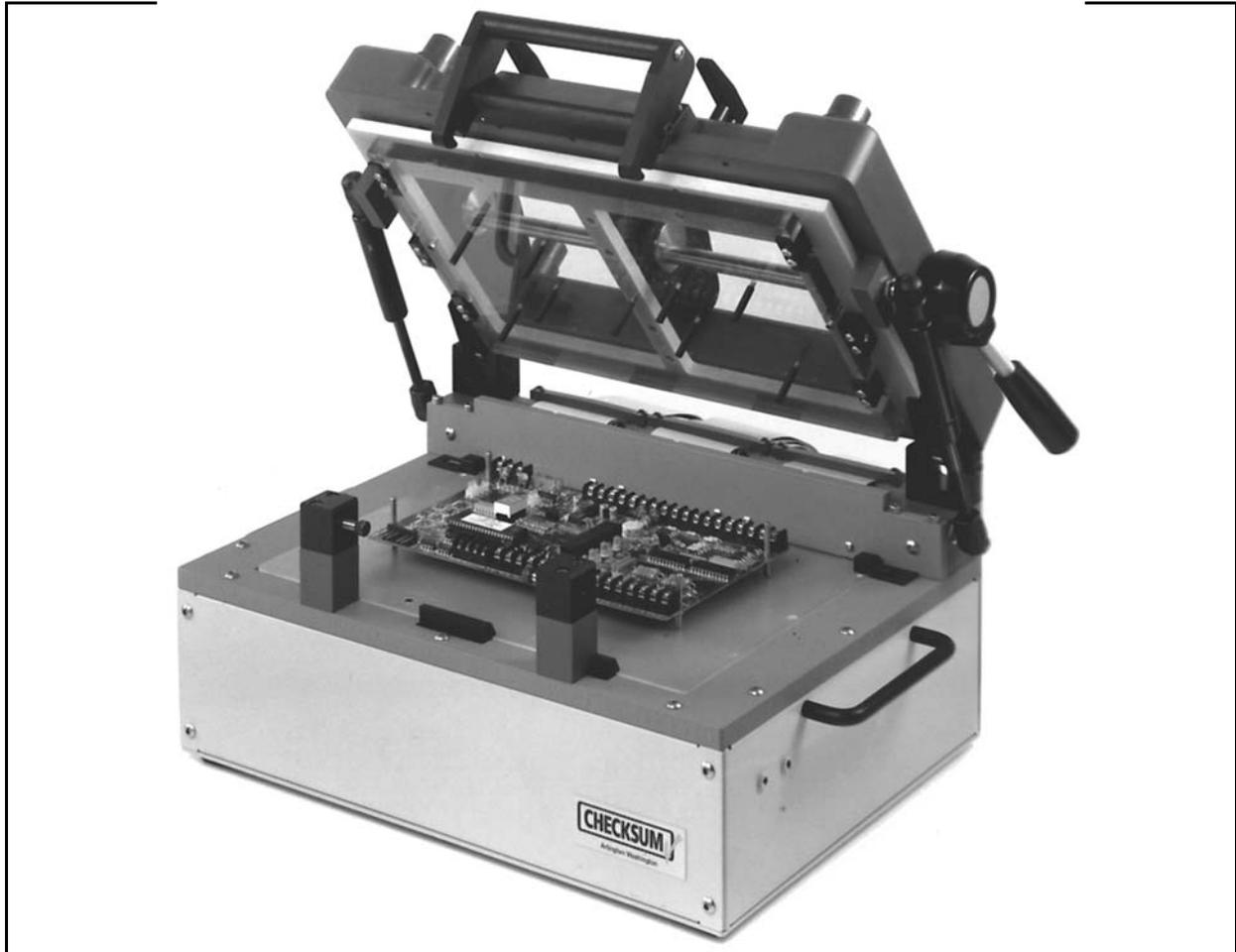
*Figure 1 - Model TR-5-600-QC Fixture System (Lid Open)*
