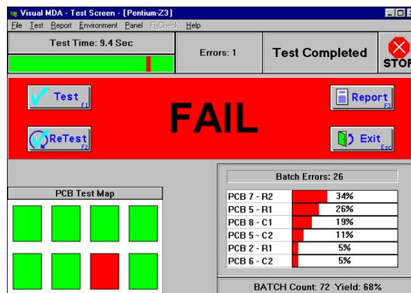
The optional system printer can be configured to output failed results automatically upon failure so they can be attached to the UUT to aid in repair. A front panel key can also be used to obtain a test report. Reports can be configured to include only information important to you.
