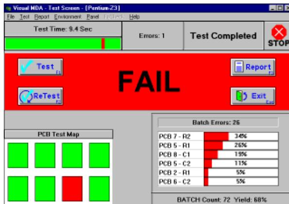
The operator can then choose to ReTest, or move to the next UUT. Most users configure the system to automatically print out a test report of component failures on the system printer if the UUT fails. The operator then attaches the failure report to the bad UUT, and sends it off for repair. The next UUT is then put into the fixture and the process starts over again. This simple operation cycle is easy to use by unskilled operators.
