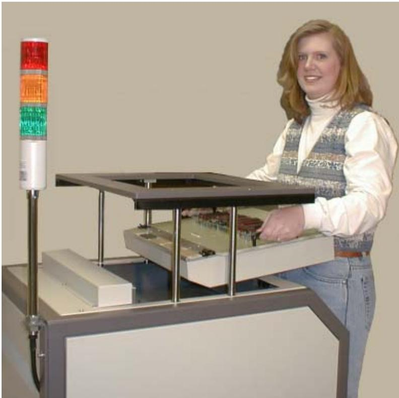
external sense (4-wire Kelvin measurements), and in conjunction with multi-point guarding to isolate individual components. Guard currents up to 100mA are available. Up to 16 distinct measurement and stimulus functions can be active during a single measurement.
