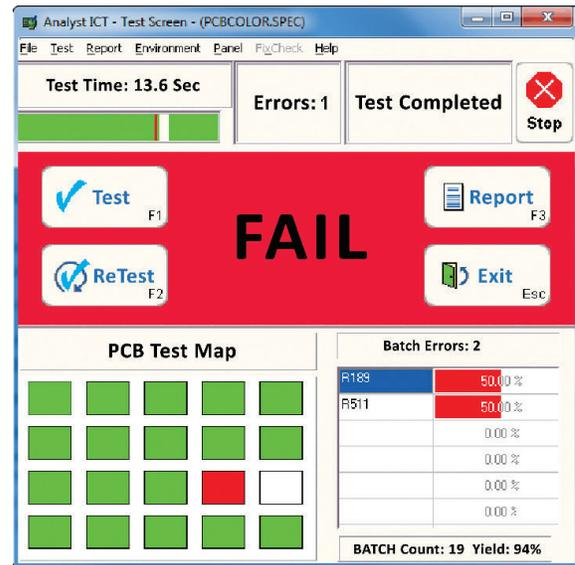
process starts over again. This simple operation cycle is easy to use by unskilled operators. Paperless repair is also possible including built-in serial number tracking. The system can be set up to halt on each failure if you would like your operators to be able to repeat steps, or repair the UUT as faults occur.
