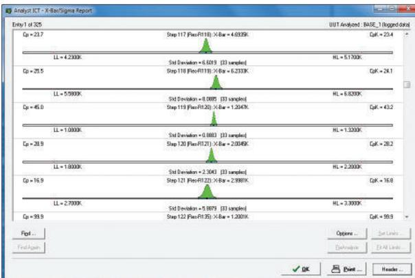
While this information can be used to monitor process measurements, it is more often used to help fine-tune test program tolerances. By observing the data, even with a relatively small programming sample size, it is practical to set control limits that are applicable to a wider range of UUTs.
