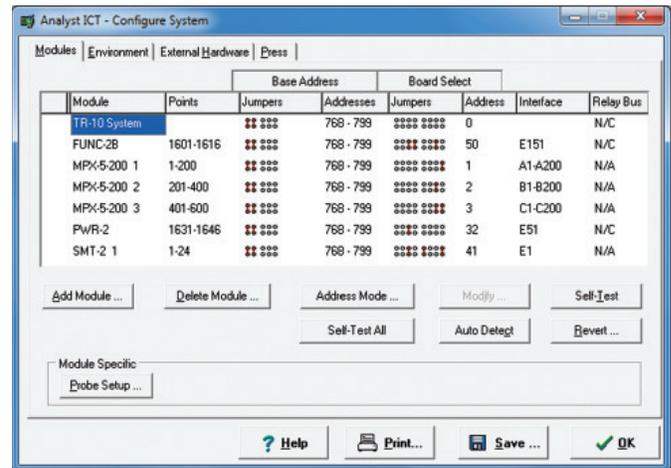
Older modules used base address only selection. The older module base addresses must have unique, non-overlapping ranges. Newer modules have base address and secondary address selections. With newer modules, the base address must all be the same. The secondary address selections must all be unique. The expected address jumpers are shown and must match the actual module jumpers.
