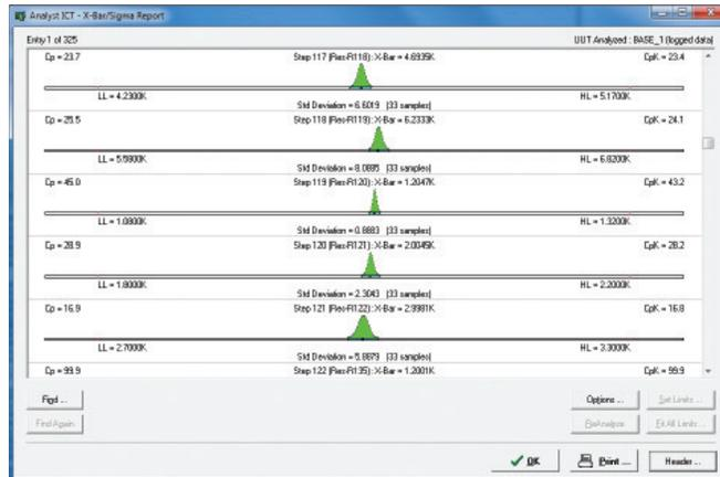
While this information can be used to monitor process measurements, it is more often used to help fine-tune test program tolerances. By observing the data, even with a relatively small programming sample size, it is practical to set control limits that are applicable to a wider range of assemblies.
