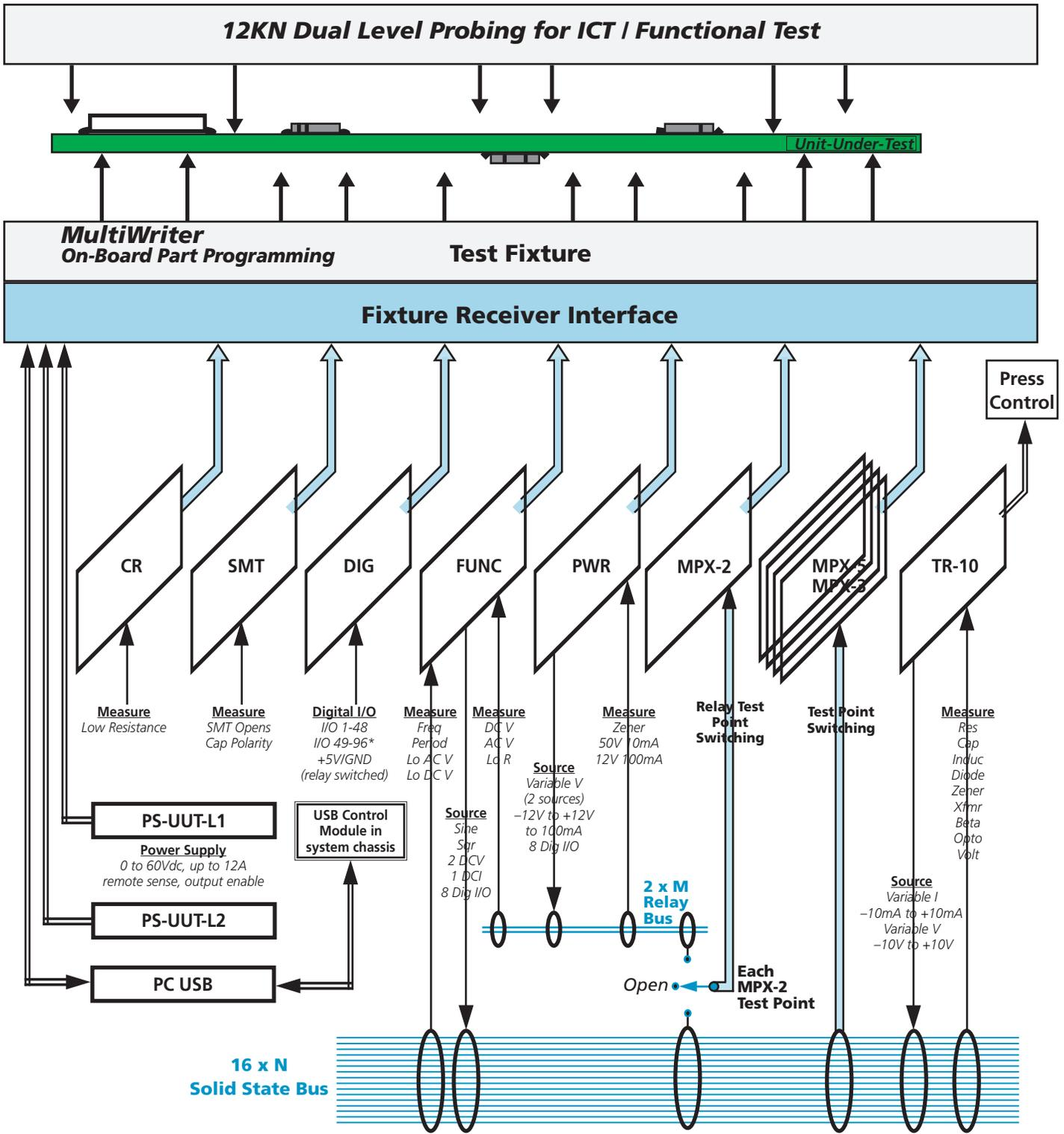
**Typical test system modules and fixture connections**
